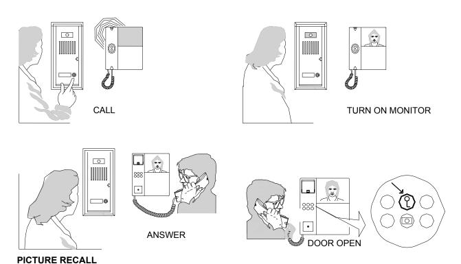
Push the button with the circle inside the square, the monitor will be working for about 30 secondos, after 10 seconds is possible repeat the operation.
