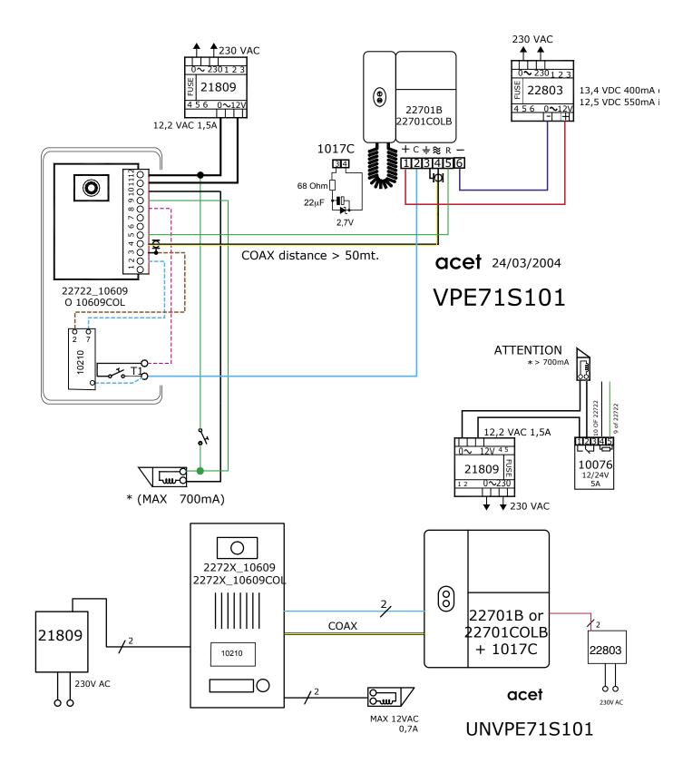
DASHED LINES MEAN CONNECTIONS MADED FROM CONSTRUCTOR.
